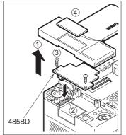
Turn off the power of the programmable controller, and mount the 485BD using the following procedure.
